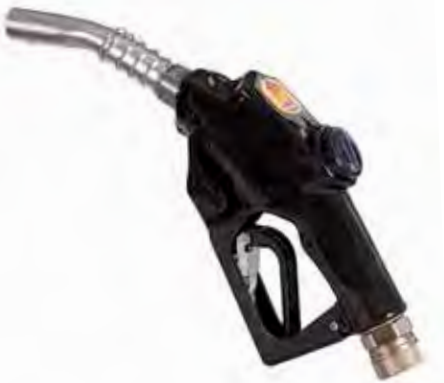
Art. 093-5215-000 Automatic nozzle "PA90" for diesel fuel transfer Flow rate 90 l/min Aluminium body Swivel connection F 1"
