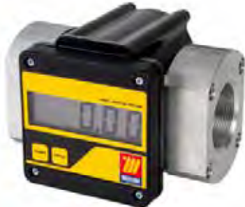
Art. 092-5150-000 Digital flow meter with gears MGE-400 min-max flow rate 15-400 l/min
