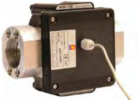
Art. 092-5170-250 Mechanical pulsed flow meter MGI-250 min-max flow rate 10-250 l/min nr. 11 pulses/liter
