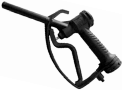
Art. 093-5199-000 Manual plastic nozzle "MP120" for diesel fuel transfer Flow rate 120 l/min Plastic body Swivel connection F 1"
