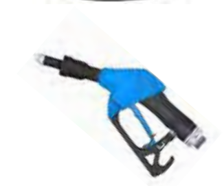
Art. 099-5220-000 ZVA Automatic nozzle for AdBlue® LV / Urea according to ISO 22241-1 (DEF/AUS/ARLA 32) for light vehicles < 3,5 t. With ATEX certificate (EX II 1G) Certificate Nr. SIRA 03ATEX9 487U Swivelling joint with integrated and certified flow regulator : TÜV - P-TÜ7-8113338228 ISO 22241 Complete with adaptor EW 22
