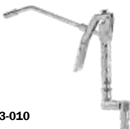
Art. 014-1083-010 Grease control gun with rigid pipe and 4-jaws coupling Length rigid pipe: 200 mm Triple-swivelling joint F 1/4"
