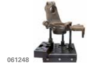
061248 Universal bearing removal support.
