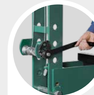
Fast and safe adjustment of the press table height, using a braked winch.
